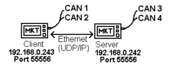
CAN-via-UDP example using two MKT-Views (2) . Note the different IP addresses ! Details in chapter 3. .
