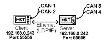
MKT-View II with four 'logical' CAN interfaces, two of them (CAN 3 and CAN 4) provided by a second MKT-View (server).
