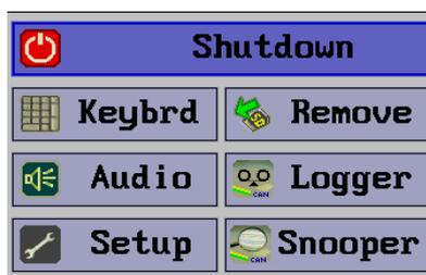
Tap on the button are labelled "Snooper", to start the CAN snooper.
